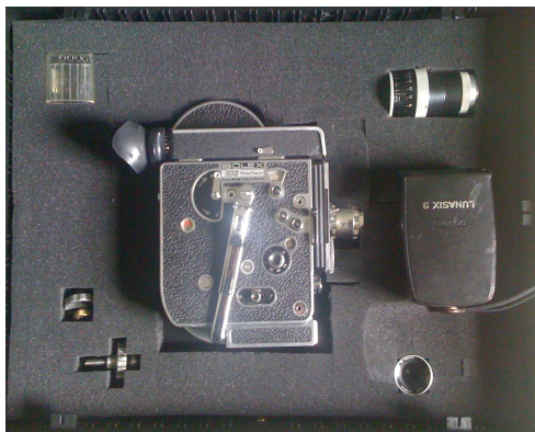
Illustration 6: clock work 16mm camera
