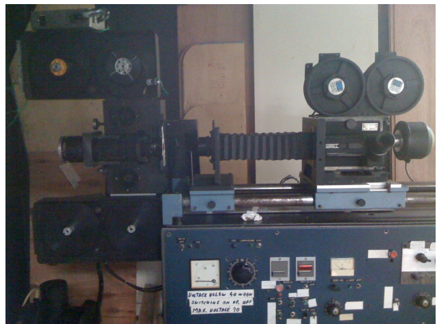
Illustration 7: Oxberry optical printer
